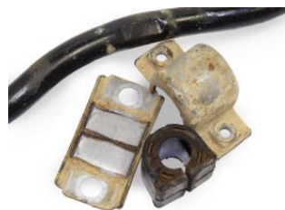
Figure 3 - the anti roll bar, brackets and the original rubber bush
