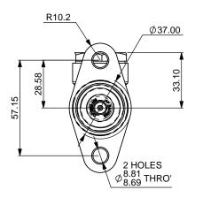
70.57 47.00 MIN THR'D DIM 37.70 -IMPORTANT FITTING OF NUT OR **CLEVIS TO FULL** EXTENT OF THREAD MAY RESTRICT PISTON TRAVEL **PUSHROD ANGULARITY** NOT TO EXCEED 4.00° INC INLET ADAPTOR-10.00
