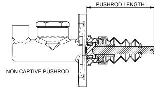
NON CAPTIVE PUSHRODS: CP2623 MASTER CYLINDER IS AVAILABLE WITH NON CAPTIVE PUSHRODS. THIS ENABLES THE REMOVAL OF THE MASTER CYLINDER WITHOUT NEED TO REMOVE THE PUSHROD FROM THE BRAKE PEDAL OR BALANCE BAR ASSEMBLY. PUSH RODS ARE AVAILABLE IN LENGTHS EQUIVALENT TO THOSE SHOWN ABOVE. PUSHROD TYPES: NCT - NON CAPTIVE PUSHROD THREADED 5/16" UNF
