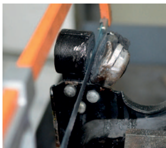
Cut original bush shoulder to enable it to be pressed out.
