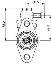
**INLET TYPE 'D'** SELECT MASTER CYLINDER WITH INLET TYPE 'B', PLUS INLET ADAPTER KIT PART NUMBER CP4623-6.
