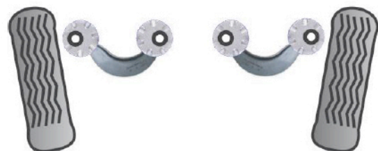
Sleeves adjusted to give maximum positive camber
