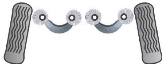
Sleeves adjusted to give maximum negative camber
