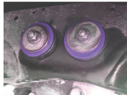
Figure 1- Fully fitted bush including washer placed near the rear of the car
